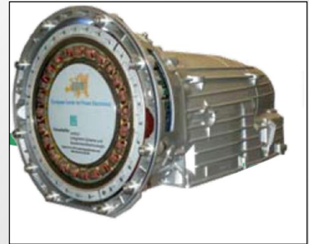
Concept for integrated Traction Inverter (Source: ECPE / FhG-IISB)
